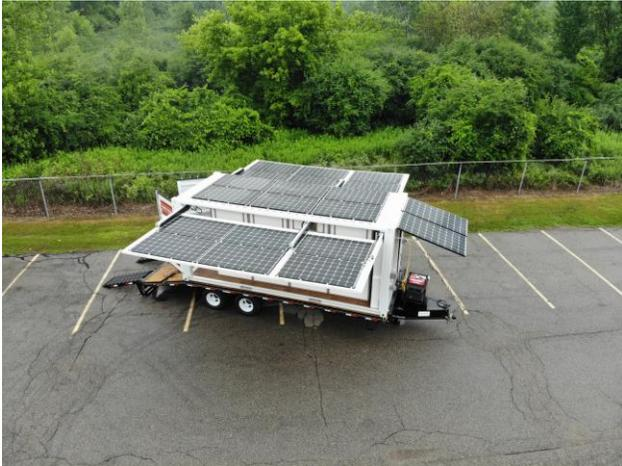
*Figure 3: Sesame Solar Turn-Key Nanogrid Fully Deployed*
