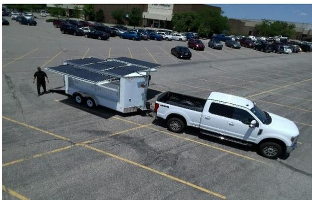
The Sesame Solar Nanogrid Solutions are very easy to deploy. Once the Mobile Broadband Access Solar Nanogrid is parked on a section of flat ground, it can be set-up in less than 15 minutes and starts producing solar power immediately. As shown in *Figure 2* below, this is all accomplished with one person. There is no need for a highly skilled or specialized operator. The solar panels stay protected and clean during transport and allow for immediate power generation once deployed. They require no
